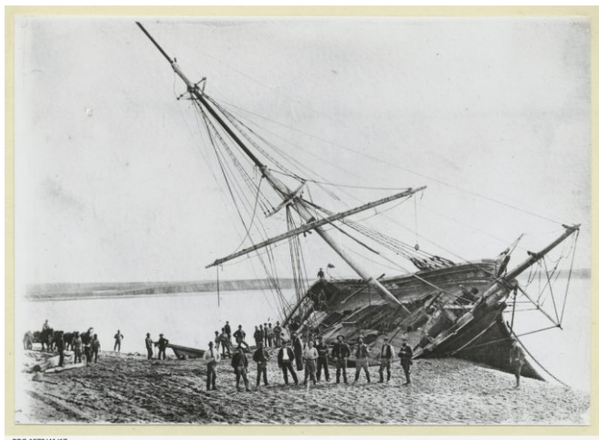
'Fairy Queen' wooden brigantine 214 tons [wooden 2 mast brigantine, 214 tons. ON45206, 111.4 x 24.5 x 13.4. Built Aberdeen Scotland, 1863. Owners: 1867 Henry Cook, registered London; March 1872 JG Punch of Sydney, registered Melbourne: May 1872 George Nipper. Wrecked at Timaru New Zealand August 27, 1873] From a volume titled 'New Zealand Owned Wooden and Iron and Steel Sailing Vessels'. https://collections.slsa.sa.gov.au/resource/PRG+1373/41/17
